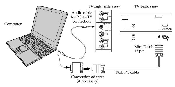
Connect a PC cable from the computer to the RGB/PC terminal on the back of the TV.
